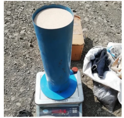
Sand Replacement method
